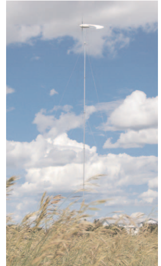
Windward Engineering 4.25kW turbine
