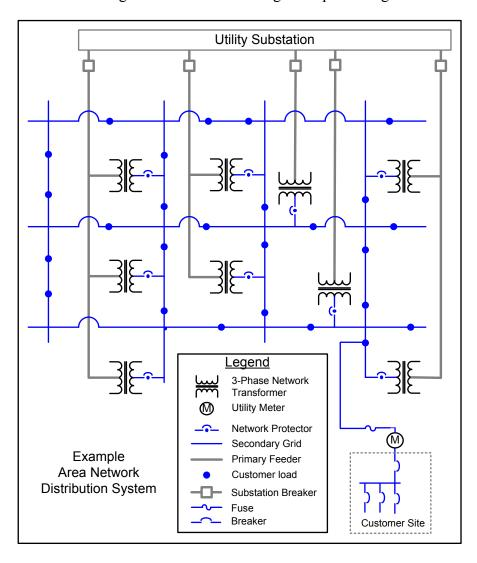
Figure 3. Example Area Network System Diagram
