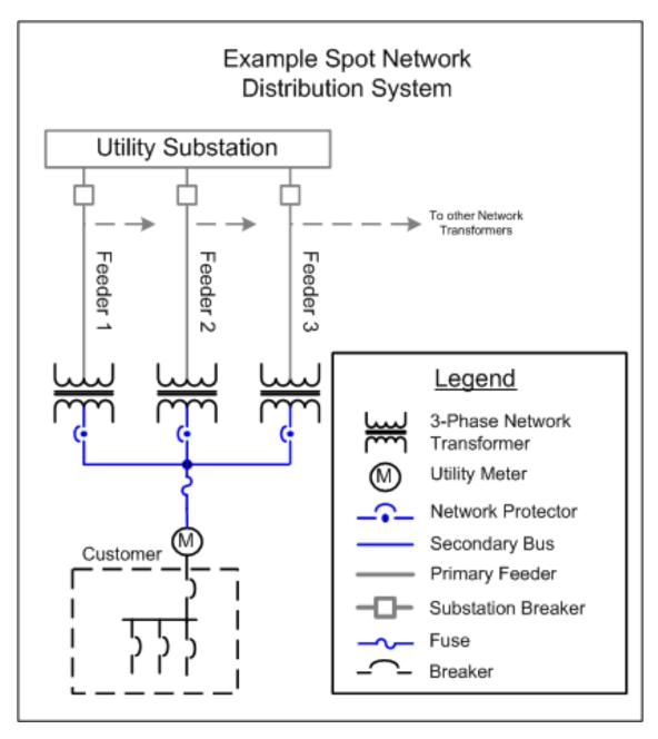
Figure 2. Typical Spot Network System Diagram
