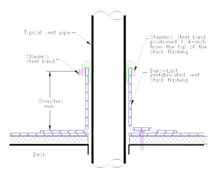
Note: Membrane attachment around the penetration will be the same as the deck membrane, max. 18—inches on center, and a minimum one plate/fastener per flashing.
