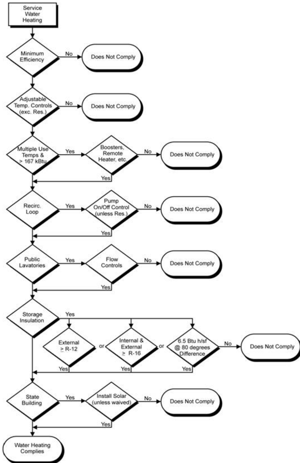
Figure 4-22 – Service Water Heating Flowchart
