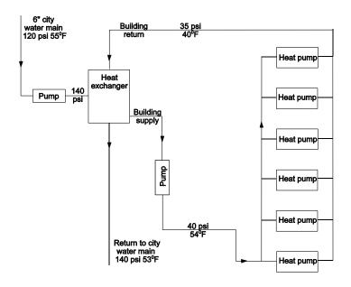
Figure 2. Schematic of Discovery Center heat pump system.
