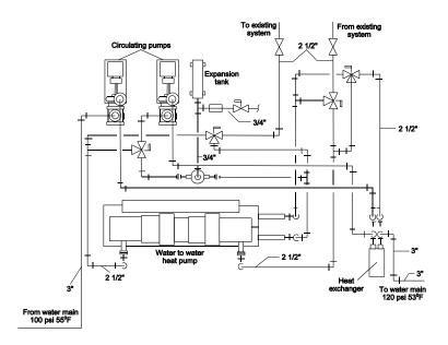
Figure 1. Schematic of City Hall heat pump system.
