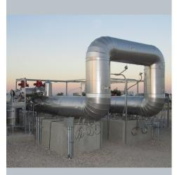
This molten salt test loop at Sandia National Laboratories' National Solar Thermal Test Facility has been used to further understand challenges related to thermal energy storage. Photo Courtesy: Sandia National Laboratories
