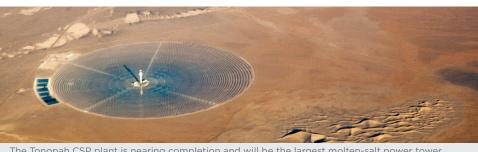
The Tonopah CSP plant is nearing completion and will be the largest molten-salt power tower CSP plant in the world, located in Tonopah, Nevada. This plant will have 8 hours of thermal energy storage, allowing it to continue to deliver power to the grid well into the night. Photo courtesy: Doc Searls
