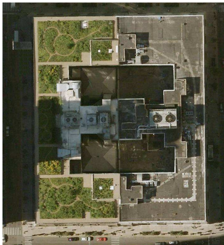
Figure 2. Roof of the building shared by Chicago City Council (left) and Cook County Council (right). The 20,000 square foot green roof, containing 20000 herbaceous plants, 100 wood shrubs, 40 vines and two trees was commissioned by Mayor Daley and completed in 2001 (10), (11)
